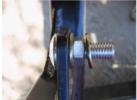
Before installing Hi Lift remove the foot off of the jack. The foot can be bolted in the backside of the antenna post using a 5/16" x 1" carriage bolt with a washer and locking nut.
