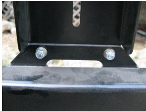
On the bottom of the antenna post use 2 @ 5/16" x 3/4" with washers and locking nuts.
