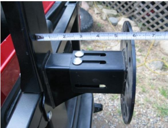
Using the measurement from the step before. Measure from the antenna post to the front side of the wheel hub. Use 2 @  $\frac{5}{16}$ " x  $\frac{3}{4}$ " carriage bolts, 2 flat washers and 2 locking nuts to tighten the top of the wheel hub down. After the top bolts are tight use 2 @  $\frac{5}{16}$ " x  $\frac{3}{4}$ " carriage bolts, 2 flat washers and 2 locking nuts to tighten the side of the wheel hub down.
