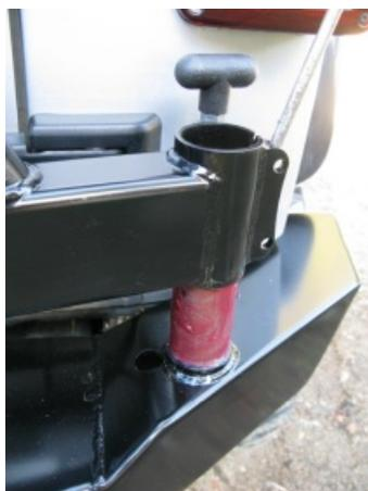
Lube the spindle on the bumper with auto or marine grease
