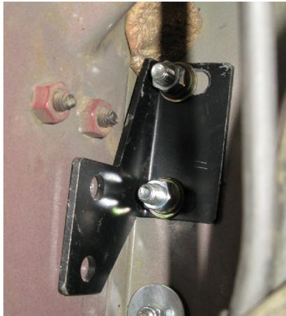
Install the latch back up plate inside the rear fender well as shown using 2 @ 3/8" flat washers and locking nuts.
