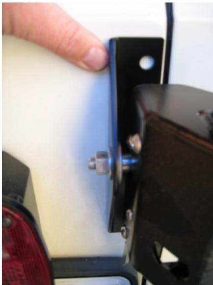
Install latch pin into the tri-l bracket. Hand tighten.
